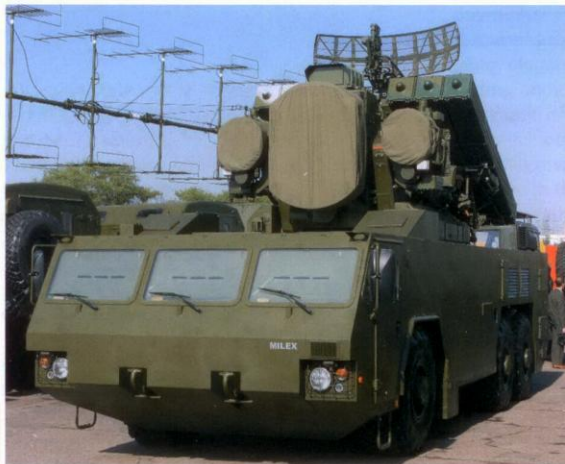
The latest version of Tetraedr's Osa-1T is based on the MZKT-69222 wheeled chassis. Miroslav Gyürösi: 1331395
