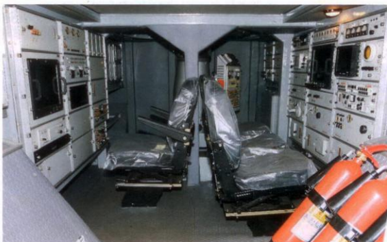
Operators' positions within the mid-section of the MZKT-69222. Miroslav Gyürösi: 1331396
